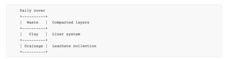
• Design: Engineered system with liners
