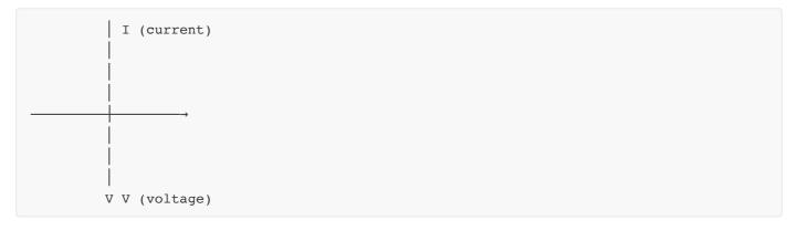
Mnemonic: "CLEAR-90" - Capacitive Load has Electrical Angle Reaching 90° (current leads voltage)
