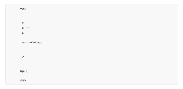
• Maximum AC power output:  $P_0 = (Vrms)^2/RL = (VCC/2\sqrt{2})^2/RL = VCC^2/8RL$
