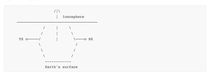
• Mechanism: Waves refracted by ionosphere back to Earth
