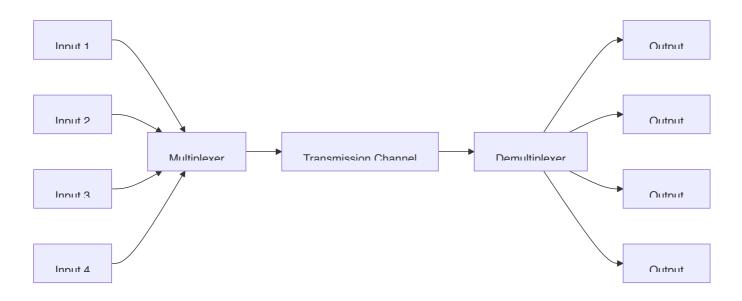
**Working:** In TDM, each input signal gets a specific time slot. The multiplexer samples each input sequentially, combining them into a single high-speed data stream. At the receiver, the demultiplexer separates the stream back into original signals based on timing.
